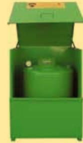
The containers, used to collect and stockpile used oils, have two inlets; one is used for loading diam. 320, it is furnished with inner grid that allows the dripping of the filters, the other of 2" x 2" is furnished with cap for collecting used oils. The mechanic level indicator is visible from the outside. There are two versions, one is for the interior (cod. SROEI-500), the other is for the exterior (cod. SROEE-500). The latter is furnished with cap with gas pistons to lift itself.
